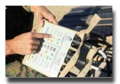
Gunnery Sgt. Andrew Suthers, the operations chief for the Infantry Officer Course in Quantico, Va., explains a color-coded light system on the Solar Portable Alternative Communications Energy System at the Combat Center Dec. 13, 2010. The SPACES is designed to tactically charge batteries and run communications equipment in remote areas such as Afghanistan. Photo: Sgt. Heather Golden
